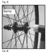
Disassemble the bearings
